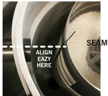
Figure 6. Align the Eazy seam to the centre of the overflow pipe.
