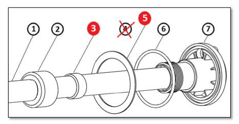
**Replacements:** The new gaskets and quartz sleeve module will work with older units and older quartz sleeve modules.
