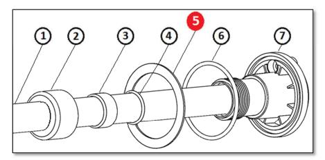
On March 16<sup>th</sup> 2018, the product line implemented another product improvement. In addition to the flat gasket, the compression fitting Gasket/O-Ring combination was replaced by a **taller gasket (PN# 960471)** and removing the O-Ring. The previous gasket measures 5/8" in height and the new gasket measures 3/4" in height.
